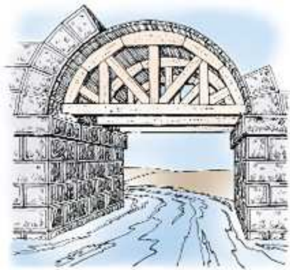
Timber frame supporting the stones of an arch. Once the central keystone was in place, the arch could support itself and the wood was removed.
